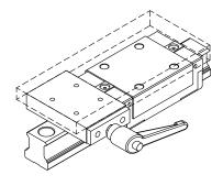
Use a connecting board to combine clamp and block. Then it's possible to locate and lock the block
